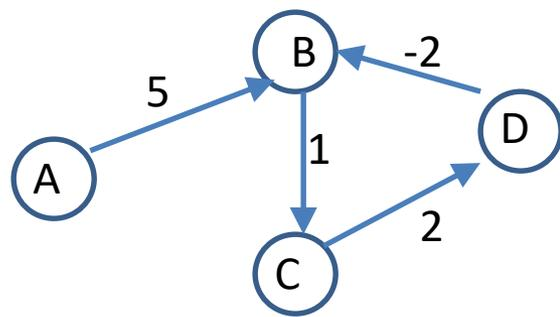
the cheapest path from A to B has cost 5, from A to C has cost 6 and from A to D has cost 8. Problems occur if the weights on the edges of a cycle sum to a negative number. Such a "negative-cost cycle" prevents there from being minimum cost paths.
